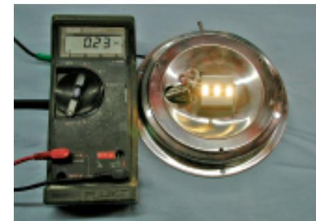
The light's amperage draw was considerably less than that of the incandescent bulb it replaced, which drew 1.49 amps.
