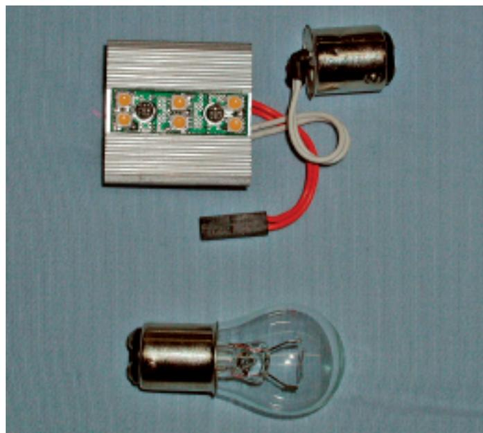
The Sensibulb LED light (top) measures a little more than 1-1/4 inches square. Below is a traditional filament bulb for size comparison.
