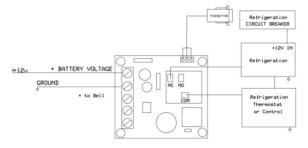
CONNECTING LOADS AFTER LOW VOLTAGE ALARM: Once activated, the Normally Open and Common contacts are connected. A load up to 30 amps may be turned on using these connections. Below is an example of such a circuit. Your own creativity is the only limit!
