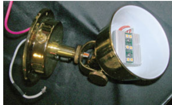
The Sensibulb's LED crystals are mounted in a patented heat sink.
