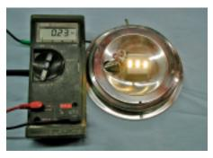
The light's amperage draw was considerably less than that of the incandescent bulb it replaced, which drew 1.49 amps.
