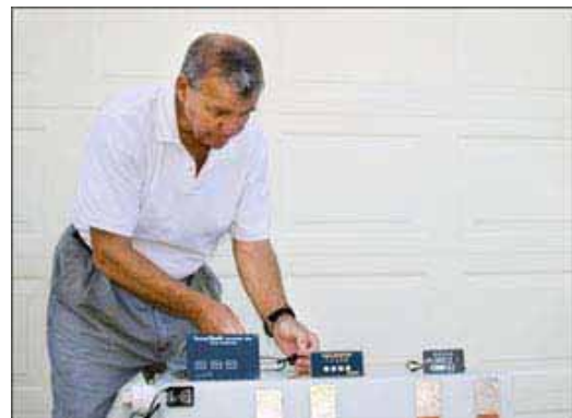
Whether it's a holding tank, a fuel tank, or a freshwater tank, keeping tabs on your tank levels is imperative. Practical Sailor testers put five tank sensors, mounted externally, to the test. Above, left to right, are the SensaTank Marine 100, the Raritan Tank Monitor, and the Scad Solo Profile Series monitor.
